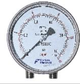
Nominal Size : 100, 150 mm Compliance to latest EN837-3 Std. ranges : 0 to 250 mmwc...10 kg/cm<sup>2</sup> Static pressure max upto 40 Bar Also available with contacts Protection to IP67 Accuracy class ±1.6% FS Stainless steel casing Dry or liquid filled version
