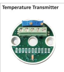
Solder Jumpers for : Span, Zero, Upscale/down Scale Output Range 4~20 mA/20~4 mA for selection Multirange : 8 SPAN ranges, 25 to 600C° / 45 to 1080 F° 4 ZERO ranges, -100 to +70 °C / -148 to +158 °F Accuracy : 0.1% temperature linear 4~20
