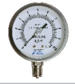
Nominal Size : 63 mm Compliance to latest EN837-1 Std. ranges : 0 to 0.6 kg/cm<sup>2</sup>...700 kg/cm<sup>2</sup> Overload capacity upto 130 % of FSD Accuracy class  $\pm$ 1.6% FS Stainless Steel Casing Dry or Liquid Filled Version Socket to case : TIG Argon Welded
