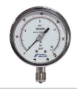
Nominal Size 100 and 150 mm Compliance to latest EN837-1 Std. ranges : 0 to 0.6 kg/cm<sup>2</sup>...700 kg/cm<sup>2</sup> Overload capacity upto 130 % of FSD Protection to IP67 Accuracy class  $\pm$ 1.0% FS Stainless Steel Casing Dry or Liquid Filled Version External Zero adjustment (Optional) Socket to case : TIG Argon Welded CE Marking as per PED 97/23/EC
