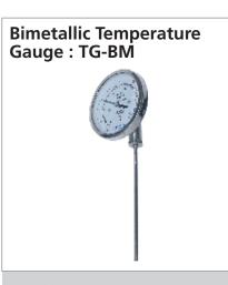
Nominal Size :100 and 150 mm Compliance to latest EN13190 Std. Ranges : -20°C to 400°C Overload capacity 110 % of FSD Protection to IP67 Accuracy class : Tolerance class 1 as per EN 13190 High repeatability, low hysteresis Stainless Steel Casing Dry or Liquid Filled Version External Zero adjustment (Optional)
