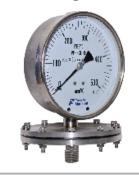
Nominal Size : 100, 150 mm Compliance to latest EN837-3 Std. ranges : 0 to 250 mmWc...6000 mmWc Overload capacity upto 125 % of FSD Protection to IP67 Accuracy class ±1.6% to 2% of FS Stainless Steel Casing Dry unfilled version Socket to case : TIG argon welded
