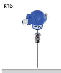
No. of Elements : Simplex / Duplex Element Type : PT-100 Range : -200 to 450 Deg. Cel.
