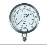
Nominal Size :100,150,200 and 250 mm Compliance to latest EN837-1 Std. ranges : 0 to 0.6 kg/cm<sup>2</sup>...700 kg/cm<sup>2</sup> Overload capacity upto 130 % of FSD Protection to IP67 Accuracy class  $\pm$ 1.0% of FS Stainless steel casing Dry or liquid filled version External zero adjustment (optional) Socket to case : TIG argon welded CE marking as per PED 97/23/EC
