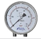
Nominal Size : 100, 150 mm Compliance to latest EN837-3 Std. ranges : 0 to 250 mmwc...10 kg/cm<sup>2</sup> Static pressure max upto 100 Bar others on request Also available with contacts Protection to IP67 Accuracy class ±1.6% FS Stainless steel casing Dry or liquid filled version
