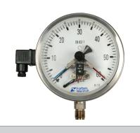
Nominal Size : 100 and 150 mm Compliance to latest EN837-1 Std. ranges : 0 to 0.6 kg/cm<sup>2</sup>...700 kg/cm<sup>2</sup> Overload capacity upto 130 % of FSD Accuracy class ±1% FS (contact accuracy 2.5%) Stainless Steel Casing
