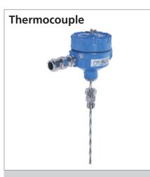
No. of Elements : Simplex / Duplex Element Type : J/K/N/R/S/B/T/E Range : Please Specify to Select suitable Element Type Hot Junction Type : Grounded / Un-Grounded Accuracy : Class I / Class II ( As per IEC-584.2 / ANSI MC 96.1) Wire Configuration : 2 Wire (SIMPLEX) / 4 Wire (DUPLEX) Sheath Material : SS316 / Other's on request Sheath Dia. : 6 mm / Other's on request Total Stem Length ( L) : As per customer requirement.
