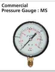
Nominal Size : 40, 50, 63, 100 and 150 mm Compliance to latest EN837-1 Std. ranges : 0 to 0.6 kg/cm<sup>2</sup>...700 kg/cm<sup>2</sup> Overload capacity upto 130 % of FSD Accuracy class ±2% FS Draw Steel With black powder Coating
