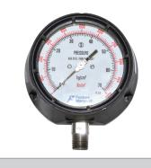
Nominal Size 115 mm Compliance to ASME - B 40.1, Grade 2A Std. ranges :0 to 0.6 kg/cm<sup>2</sup>...700 kg/cm<sup>2</sup> Overload capacity upto 130 % of FSD Protection to IP67 Accuracy class ±1.0% FS Polypropylene case with SS316L measuring system Dry or Liquid Filled Version
