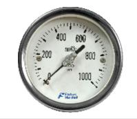
Nominal Size : 100, 150 mm Compliance to latest EN837-3 Std. ranges : 0 to 250 mmWc...6000 mmWc Overload capacity upto 110 % of FSD Protection to IP67 Accuracy class  $\pm 1.6\%$  to  $\pm 2\%$  FS Stainless Steel Casing Dry unfilled version General Purpose Pressure Gauge : GP For Hydraulic Applications
